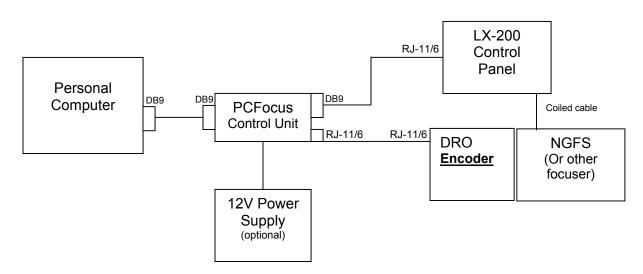
**WARNING!** Do not plug the 6-wire modular cable from the PCFocus Control Unit into anything but the JMI DRO Encoder connector or damage will likely result to the incorrectly connected equipment.
